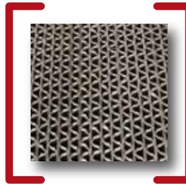
Waterjet cutting bricks are specially designed to assist in the cutting of difficult parts. Made from a unique HDPE, the bricks are manufactured specifically for the waterjet cutting industry. The bricks are designed with laminated flute pattern which minimizes splash-back while draining water and debris away quickly and effectively.
